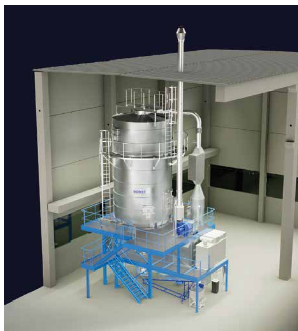
Fig. 5 Customized spray dryer plant – D600
