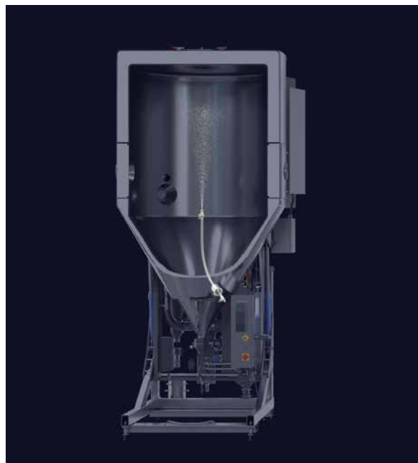
Fig. 3 Counter-current process – Two fluid or pressure nozzle
