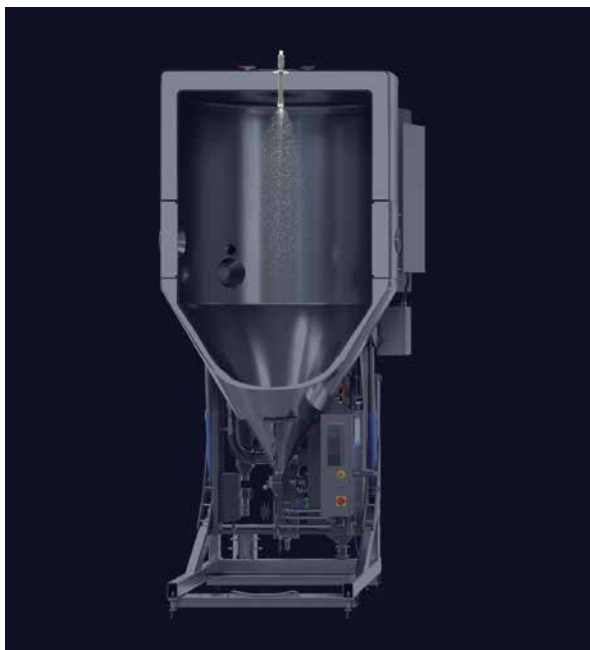
Fig. 2 Co-current process – Two-fluid or pressure nozzle
